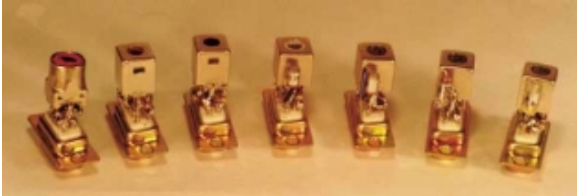
Various versions of L2 for full frequency coverage.
