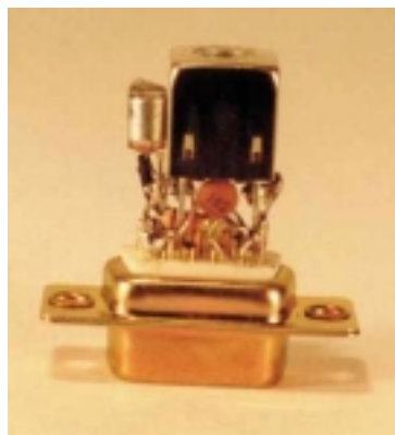
Fig.6. The audio power amplifier PCB (approximately full size).
