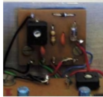
Tuning board mounted on the side of the chassis.
