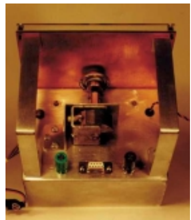
Chassis topside layout showing D-type socket for the tuning coils.
