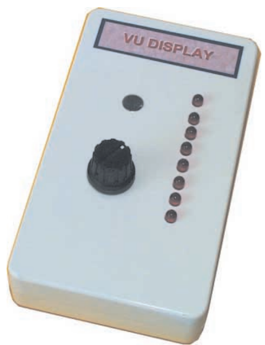
Fig.6. Adding a “diode pump” circuit to produce a simple VU Indicator.
