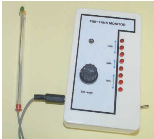
Completed Temperature Sensor module. Note the thermistor mounted in a discarded ballpoint pen barrel.
