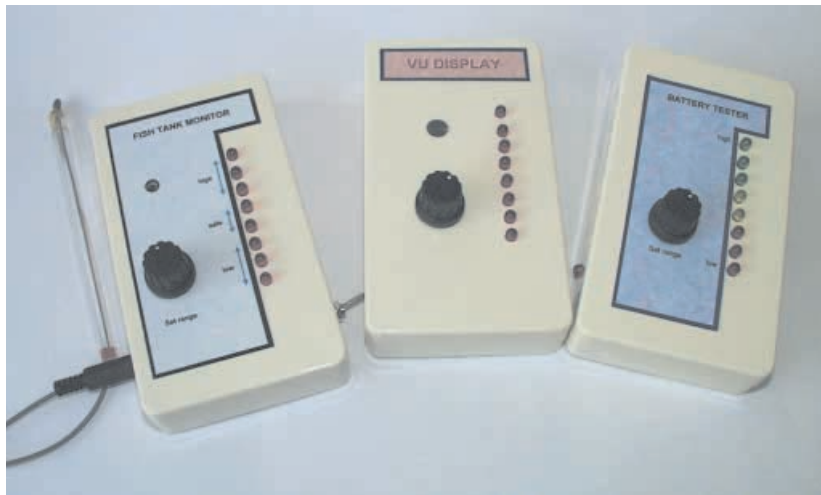
Line-up of this month's three demonstration modules: ● Temperature Sensor – Fish Tank Monitor ● VU Indicator – Volume Level Display ● Voltage Sensor – Battery Tester.
