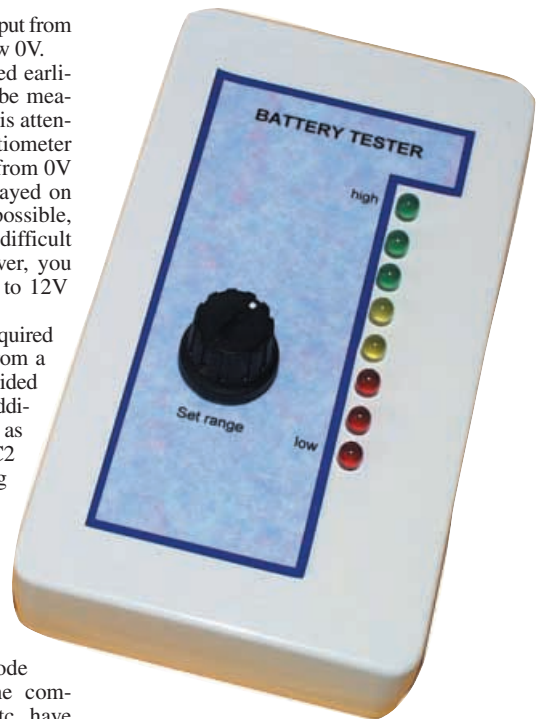
Completed prototype Voltage Sensor (Battery Tester). The I.e.d.s shown here are made up of three red (low), two yellow and three green lights.
