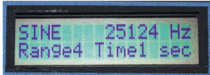
This display shows a sine wave is being generated and a frequency of 25,124Hz has been registered via range 4.
