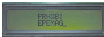
An encrypted message from the Matchbox unit (top) and its decoded meaning (lower).
