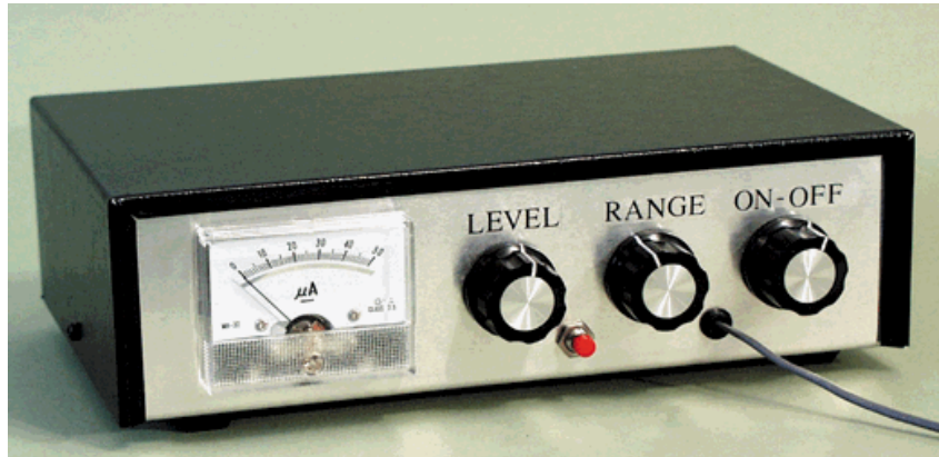
Finished unit showing front panel layout and lettering. Note the phototransistor/diode light sensor is attached to the free end of the screened cable.
