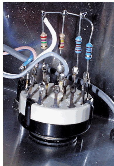
Fig.4. Camera Shutter Timer stripboard component layout, inter-wiring and details of breaks required in the underside copper strips. (Right) Mounting the Range resistors directly on the switch tags before it is fitted in the case will help with the final wiring.
