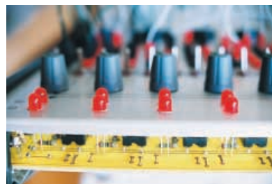
Edge-on view showing front panel and p.c.b. relationship.
