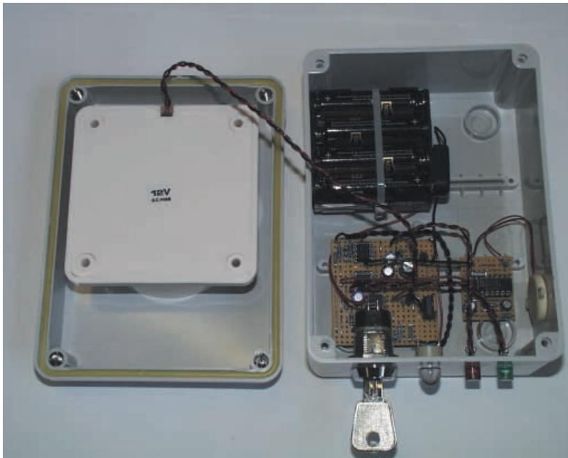
Completed Opto-Alarm system showing the main siren in the lid.
