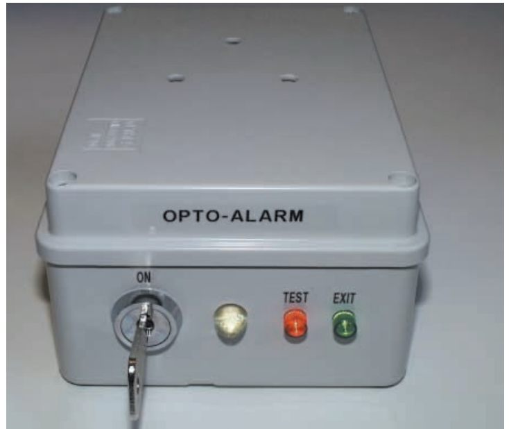
The keyswitch, light sensor and test and exit l.e.d.s mounted on a side panel of the waterproof case.
