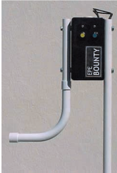
Finished control box mounted to the handle and search head shaft.
