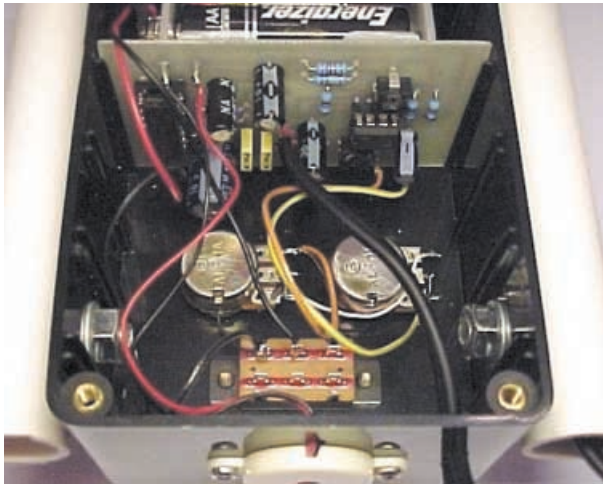
Mounting of the p.c.b., controls and sounder in the case.
