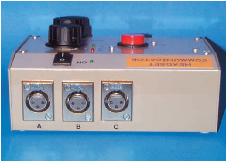
Rear panel shows the three XLR type sockets for connecting up the Slave units.
